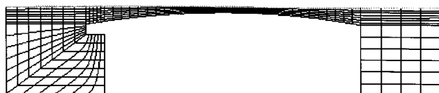
Figure 6. Representative mesh used to discretize the problem: 476 elements and 8,929 unknowns.
